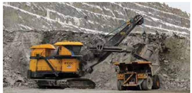
This modern haul truck and excavator illustrate a situation where exposure to whole-body vibration from vehicles occurs in the mining environment
